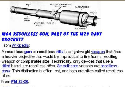
Unlike other recoilless weapons, the M29 has a firing mechanism that is integral with the propellant cartridge instead of being a component of the weapon.
